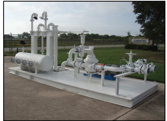
Ethanol Off-loading Skid
